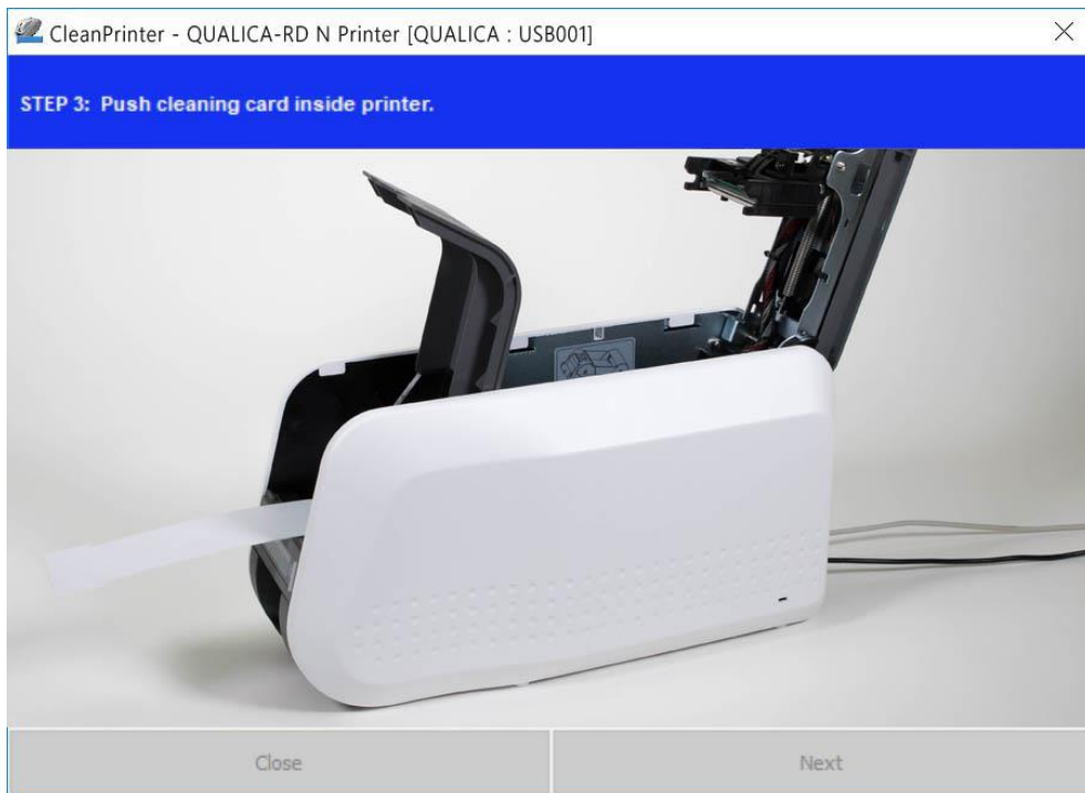
Figure 108 Printer cleaning Step 3
