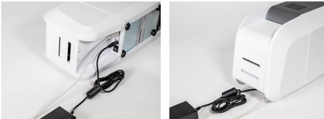
Figure 10 Dual-sided Card Printer Connection of power and USB cable
