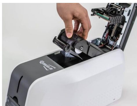
Figure 19 Installing the ribbon cartridge
