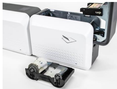
Figure 22 Loading the laminating film
