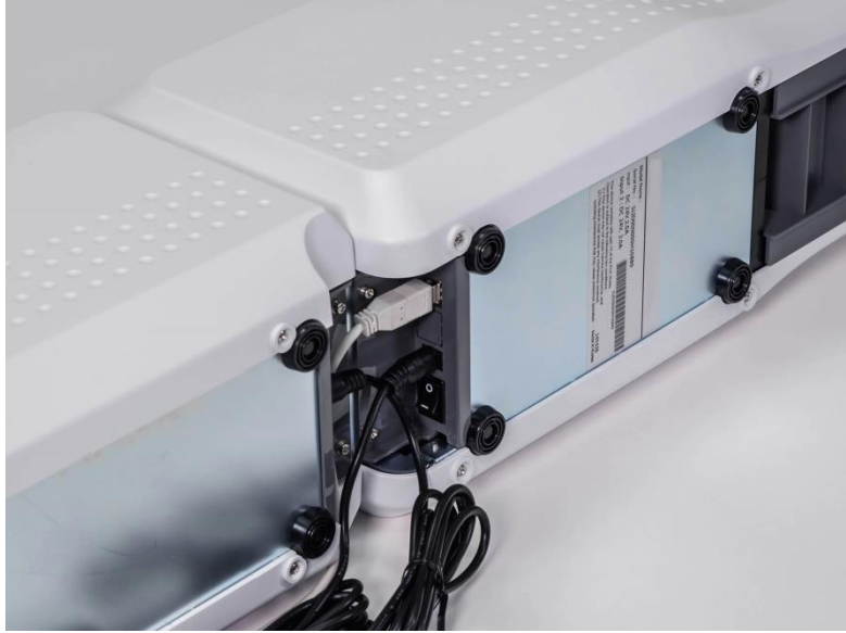
Figure 11 Laminating Card Printer Connection of powers and USB cable - 1
