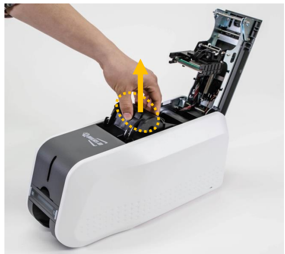
Figure 14 Take out the ribbon cartridge
