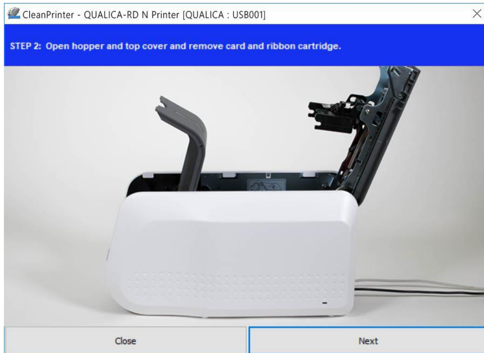
Figure 107 Printer cleaning Step 2
