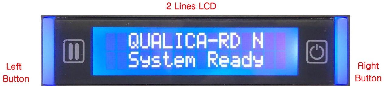
Figure 8 QUALICA-RD N Printer Display and Buttons
