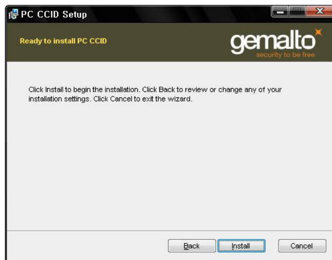
Figure 98 Installing the contact smartcard reader driver
