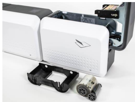
Figure 21 Take out the film cartridge
