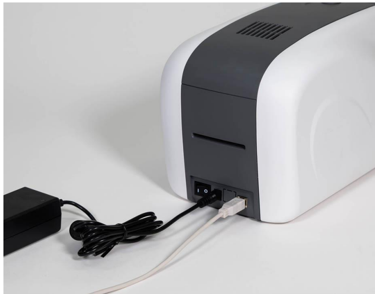
Figure 8 Single-sided QUALICA-RD 301 Printer Connection of power and USB cable
