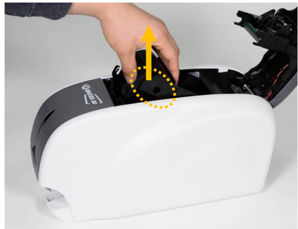
Figure 11 Take out the ribbon cartridge
