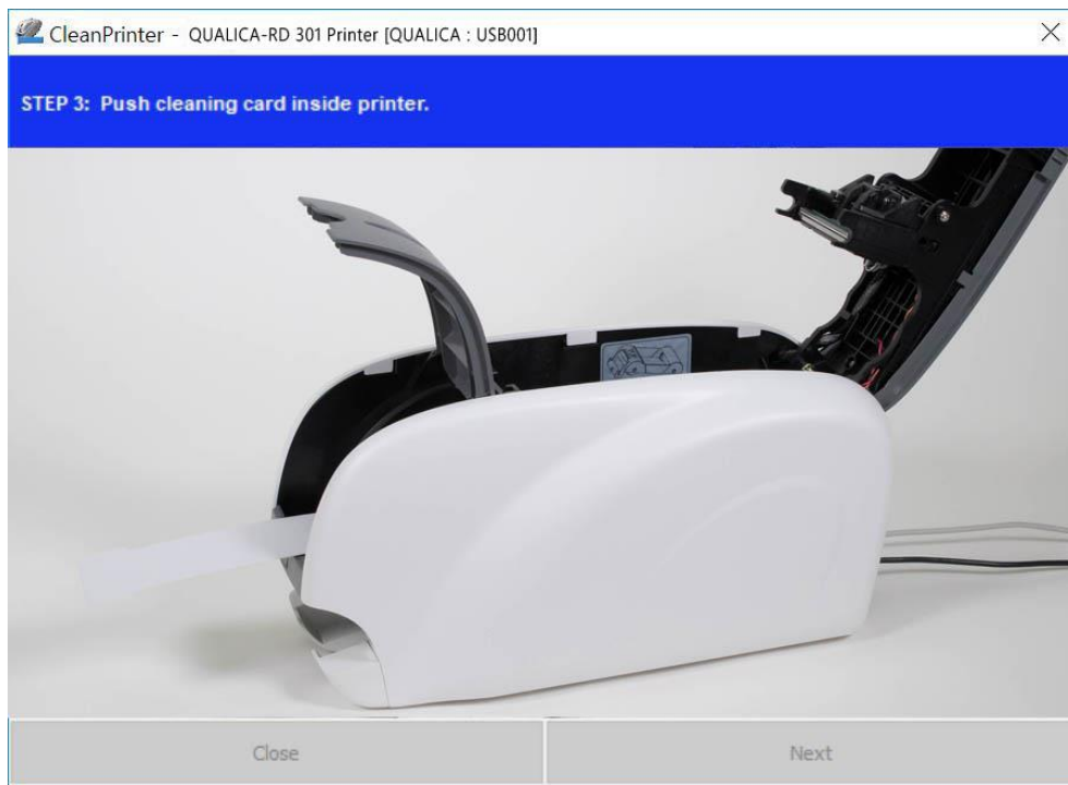
Figure 97 Printer cleaning Step 3
