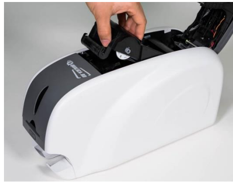
Figure 16 Installing the ribbon cartridge
