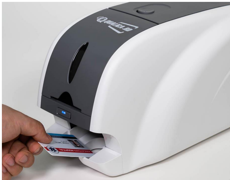
Figure 25 QUALICA-RD 301 Printer Withdrawal a card
