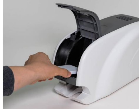
Figure 22 Loading the cards 2
