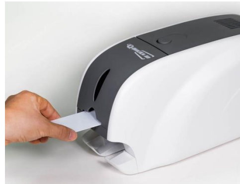
Figure 23 Loading the cards 3
