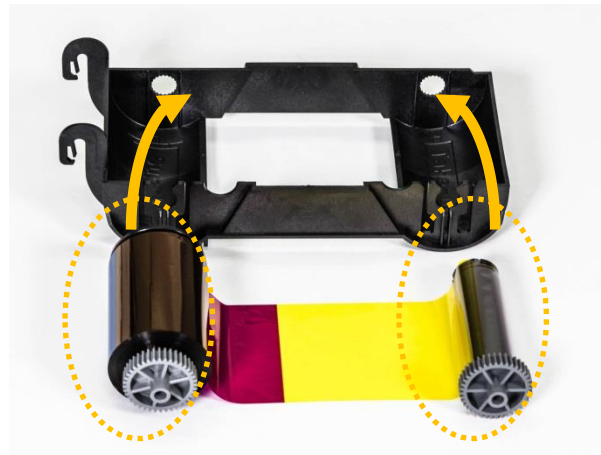
Figure 12 Loading the ribbon 1
