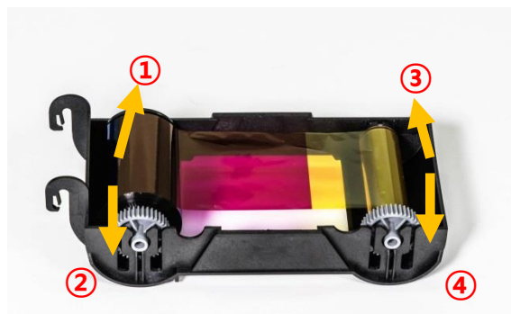
Figure 13 Loading the ribbon 2
